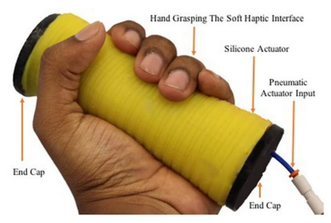
This soft-robotic device, with its variable stiffness settings, eliminates the need for multiple devices and enables effective rehabilitation of sensorimotor hand function in a single device.
