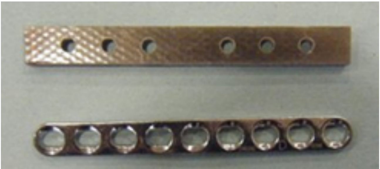
Figure 1: Representative image of composite plate in comparison to a typical metal plate used for fracture fixation.
